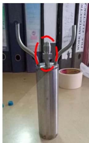
Figure 5: Male to Female Connector soldered
