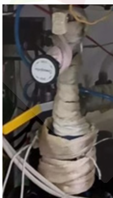
Figure 3: Precursor Bottle heated for getting vapours using Fiber Glass Tape Heater
