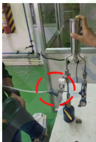
Figure 8: Evacuating the 'T' Using the Rotary Pump
