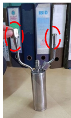
Figure 6: Swagelok Port Connectors Welded at Input-Output Tubes
