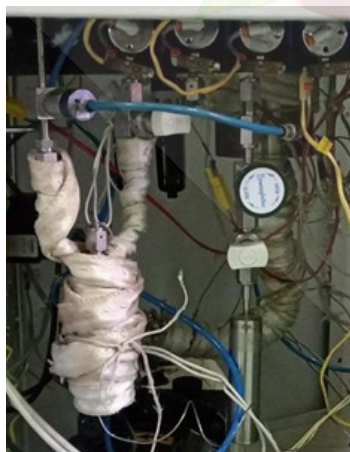
Figure 10: Bubbler is heated using the Fiber Glass Tape Heater. H 2 O is filled in S-S Precursor and is connected to the 2nd ALD Valve from right. Left Tube (inlet tube) of the Bubbler is connected to Rightmost ALD Valve (Used for Controlling the Flow of N 2 gas). Right Tube (outlet tube) of the Bubbler is connected to the Leftmost ALD Valve (Used for pulsing TTIP carried with N 2 in the Reactor).
