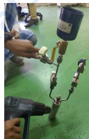
Figure 9: Hot-Air Gun Used to Transfer the Precursor in Fabricated Bubbler
