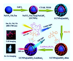
**Figure. 1:** Schematic of the preparation and structure of multifunctional mesoporous NPs containing both upconversion and magnetic nanophosphors (with an architecture of the type NaYF4:Yb,Tm@ NaGdF4) and covered with a conventional luminescent lanthanide complex (Ln-dbm) for use in upconversion and downconversion luminescence imaging and as T1-weighed MRI contrast agents. From ref. 3
